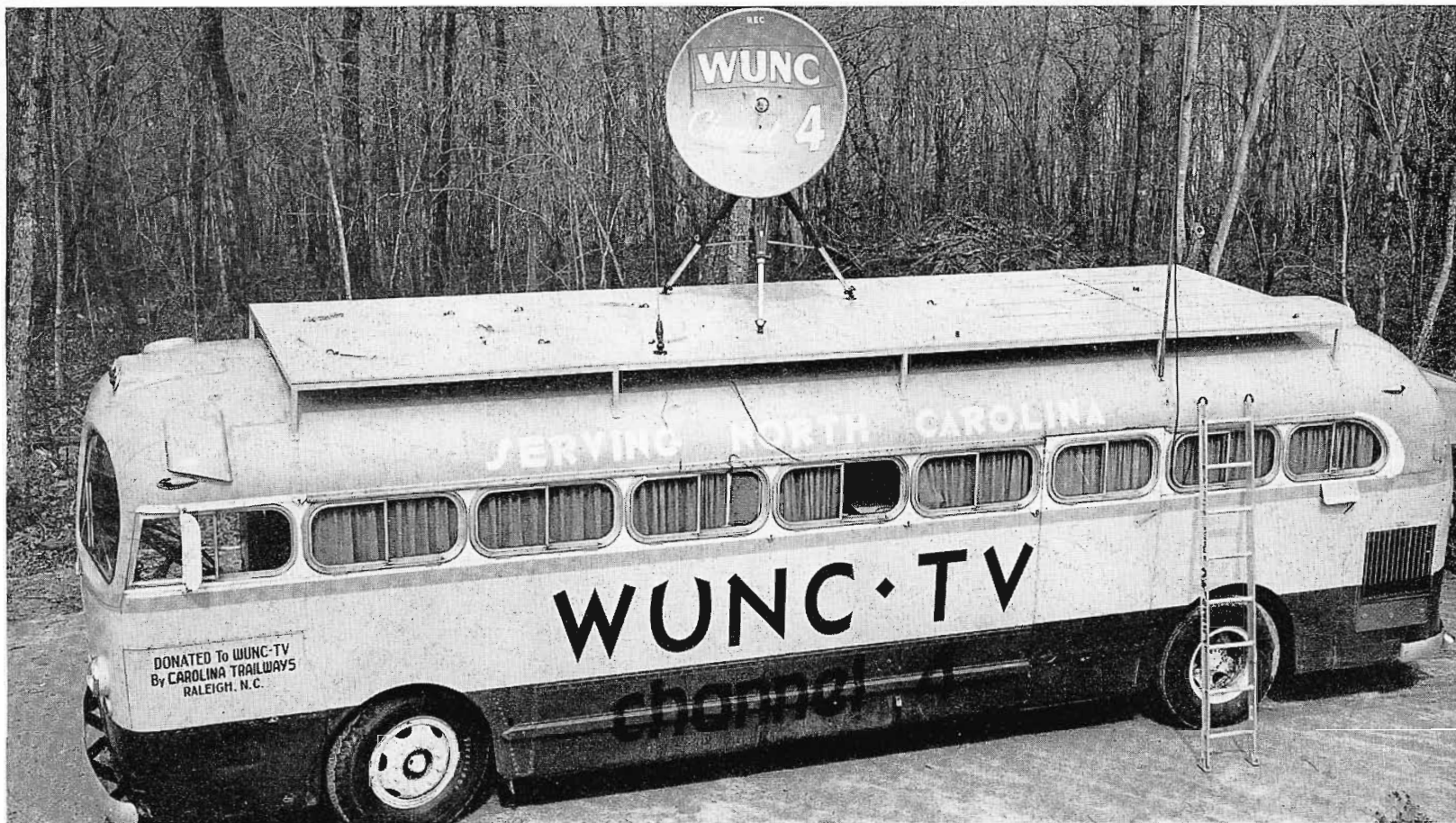
FIG. 48. WUNC-TV mobile unit for handling remote origination. Equipment includes two TV cameras, video control and audio. Also microwave relay and communication equipment.
