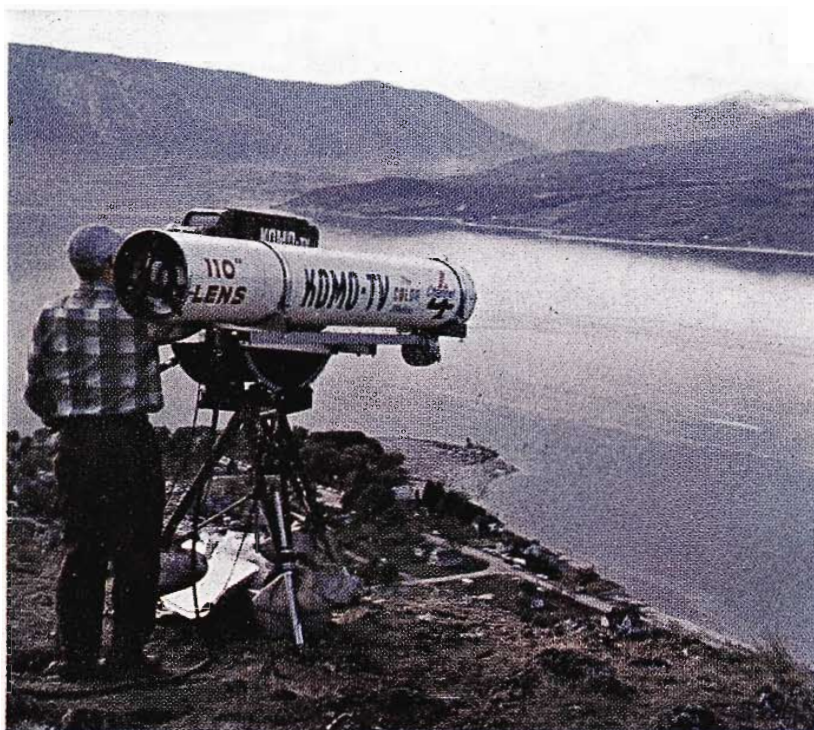
FIG. 29. Giant 110-inch sports lens in use at annual hydroplane race on Lake Chelan. This gives viewers a close-up of all action. At a distance of one mile this lens can close down on a man in the cockpit of the boat.
