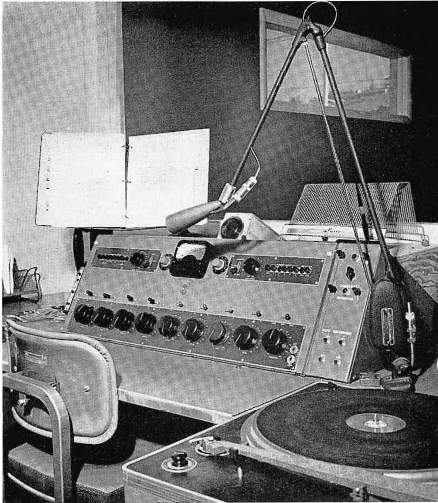
FIG. 22. Remotes, studio shows, music programs are all channeled through versatile BC-2B studio console in control room of station KUMA.
