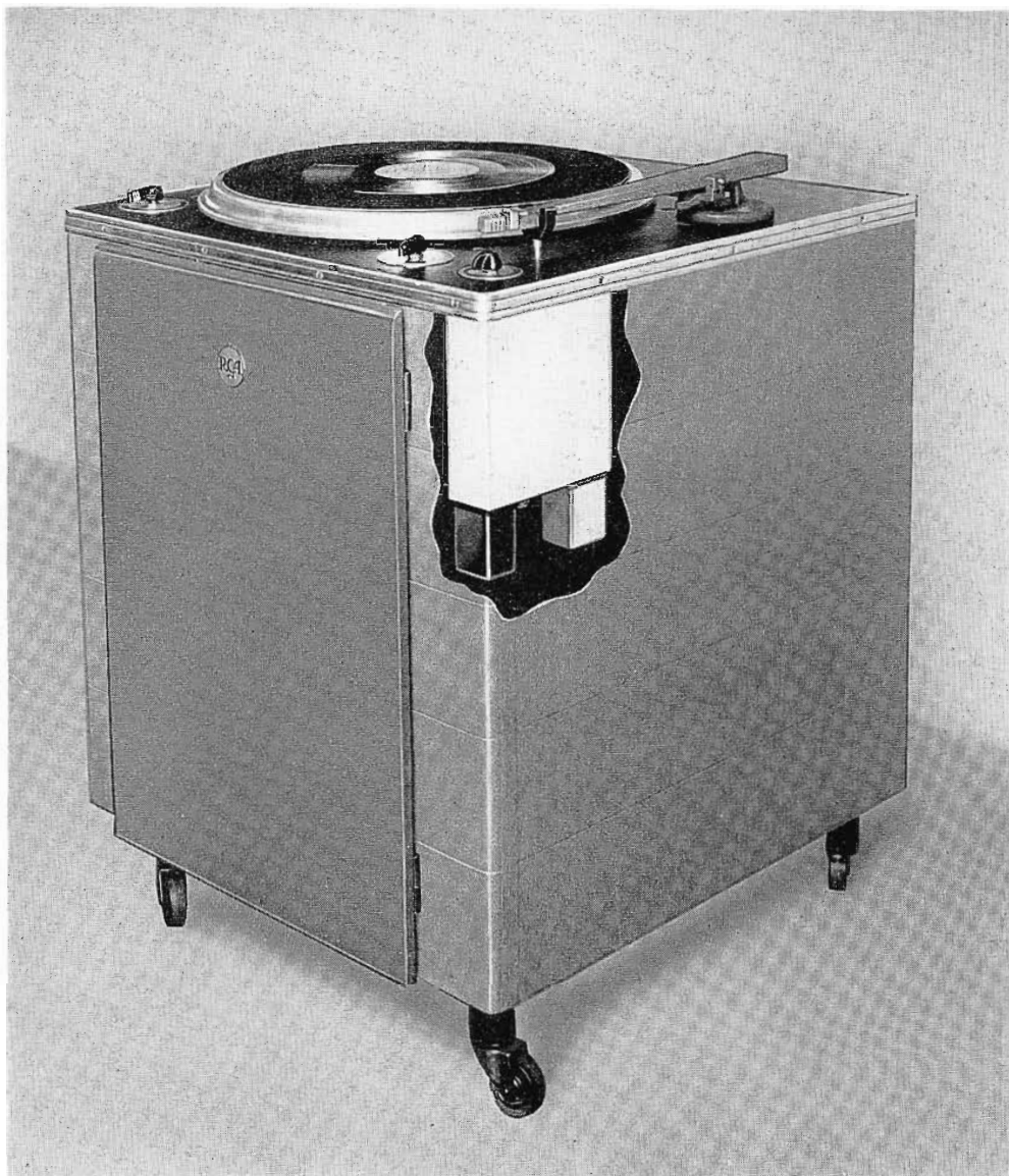
FIG. 3. This shows the BA-26A mounted in a BQ-2B Three-Speed Turntable. Observe the convenient position of the BA-26A response selector switch—next to the turntable motor switch.
