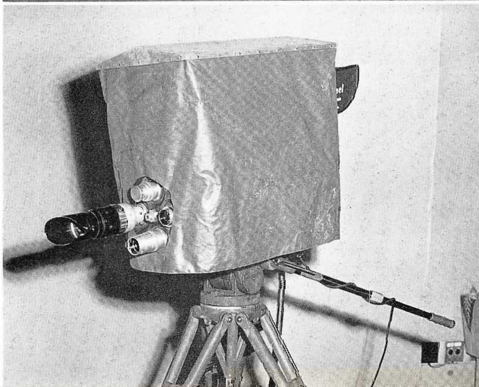
FIG. 31. TV raincoat constructed for camera. Made of a lightweight, waterproof cloth material, it provides ample air circulation and protection from inclement weather on outside remotes, yet is easily and quickly removed.
