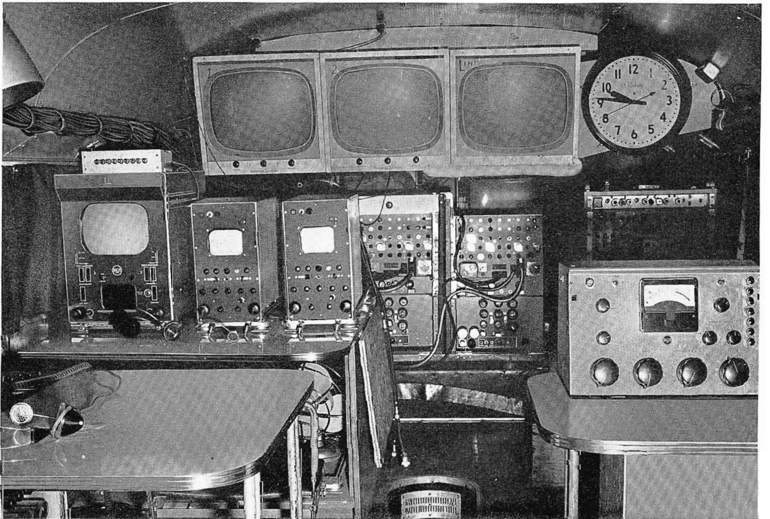
FIG. 51. Interior of WUNC-TV remote unit: left foreground, director's desk and switcher; right foreground, audio desk; left center, video control; rear, power supplies and microwave transmitter.
